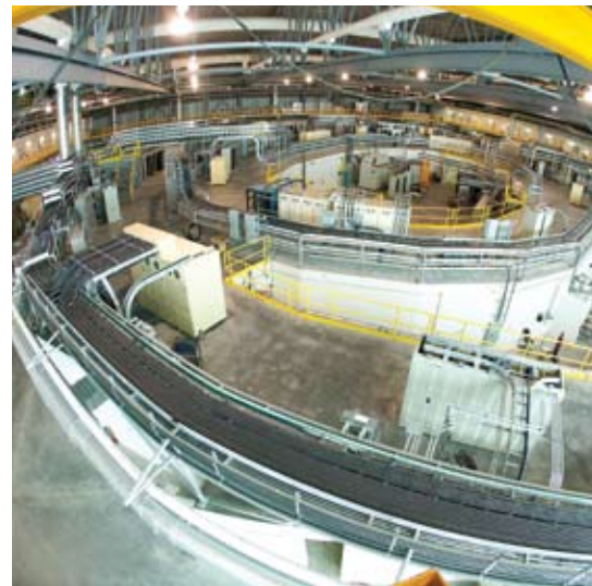
Birdseye view of CLS booster and storage rings. (Photo courtesy of Canadian Light Source Inc., University of Saskatchewan)
